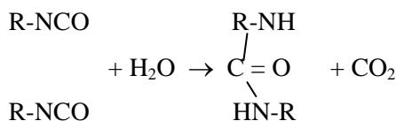
As shown the reaction leads to production of MDA and the CO<sub>2</sub> that causes foaming.
