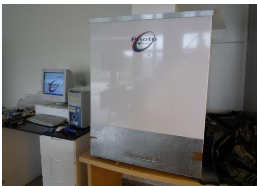
Fig 12. The photo box to analysis fat content of the salmon fillets (Original photo, Hang)
