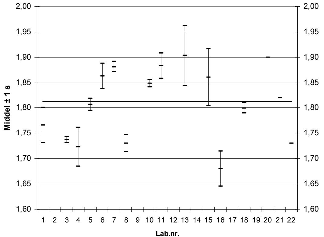
**Figur 23. Tørrstoffinnhold, prøve A**
