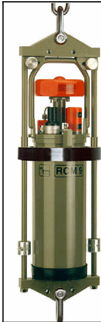
Figure 2. The Aanderaa RCM9 Doppler current meter, with turbidity sensor to the right.
