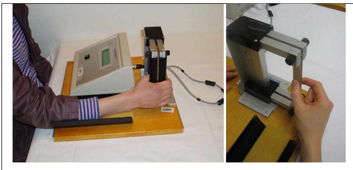
Figure 1: The instrument Grippit, grip strength to the left and pinch grip to the right.
