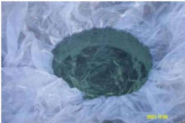
Figure 10: Water used to measure excavated volume.
