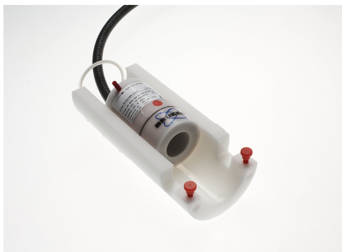
Figure 2.3: RF mouse head quadrature volume resonator Photo by Anne Herdlevær
