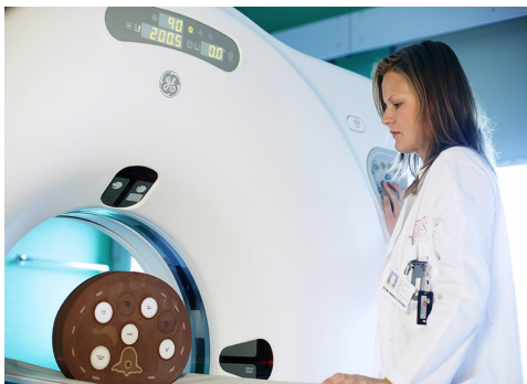
Figure 2: A custom made anthropomorphic, upper abdomen phantom specially designed for ROC studies. In the phantom are simulated liver lesions in the range 2-7 mm.
