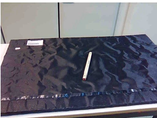
Fig. 27 Visible delamination of the fleece cover after exposure at 80°C for approximately 1 month. More of the envelope cover has lifted from the substrate than after 7 days. No further changes were observed during the rest of the ageing period.
