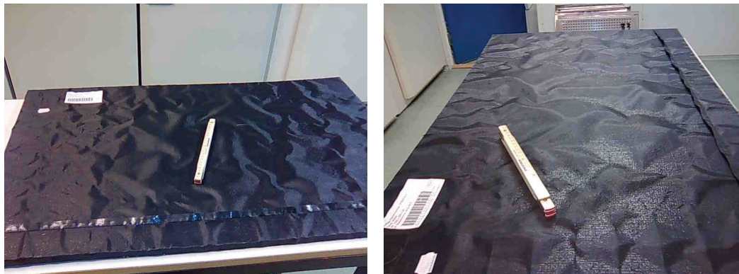
Figure 4 Visible delamination of the fleece cover after exposure at 80^\circ\text{C} for approximately 1 month.
