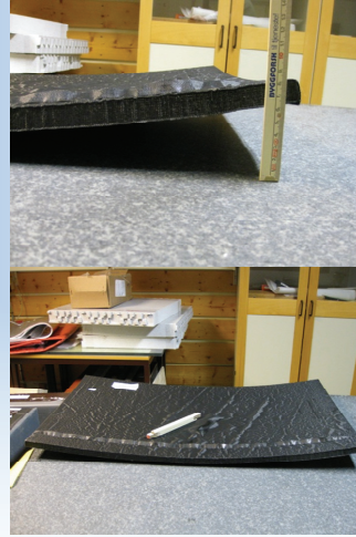
Exposed NT Build-panel, 1 month
