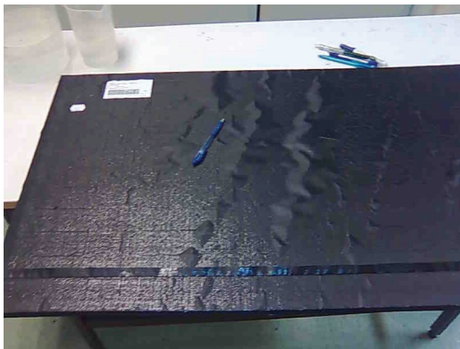
Fig. 26 Visible delamination of the outer fleece layer of the VIP envelope after exposure at 80°C for 7 days.
