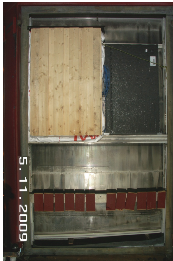
Fig. 28 Wall section of the climate simulator showing both VIPs. The exposed VIP can be seen in the top right corner, while the protected VIP is behind the weatherboards.
