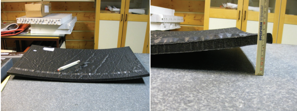
Figure 5 Uncovered panel after exposure to cyclic climate strains in vertical climate simulator for approximately one month. Some delamination of the fleece cover is visible. The panel had curved during exposure.
