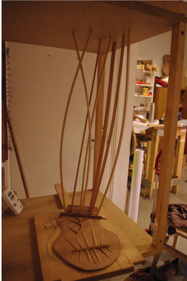
Figur 17: Liming i go-bar-deck.
