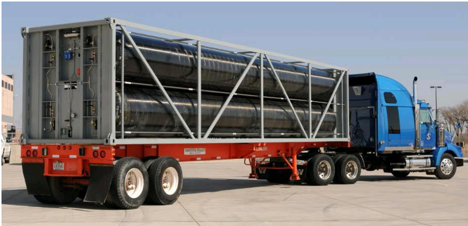
Figure 4. New type of hydrogen delivery truck [14].
