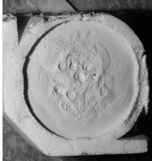
Figure 2.7: Preliminary experiment on the sublimation of dry-ice within a bed of fine particles triggered by heating through resistor treads. The image is 7 cm across. Circular gas-escape structures form.
