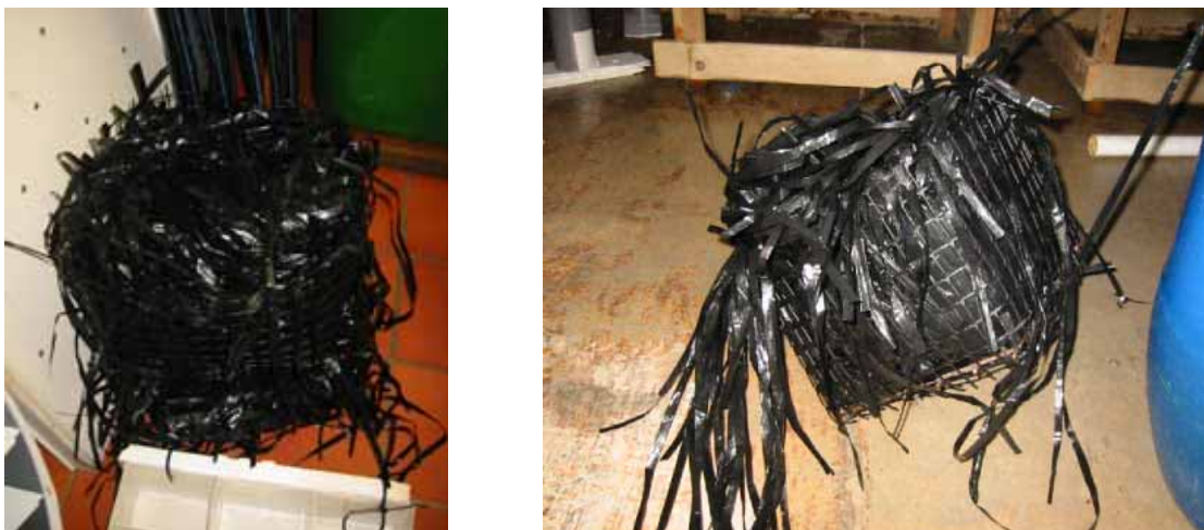
Figure 5.5. Artificial polyethylene substrate for tested for communal rearing of IV-VIII stage lobsters
