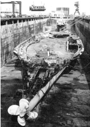
Picture 3: The Netherlands: Scrapping a ship in dry dock prevents pollution of ground and surface water with oil. ( www.greenpeace.org )
