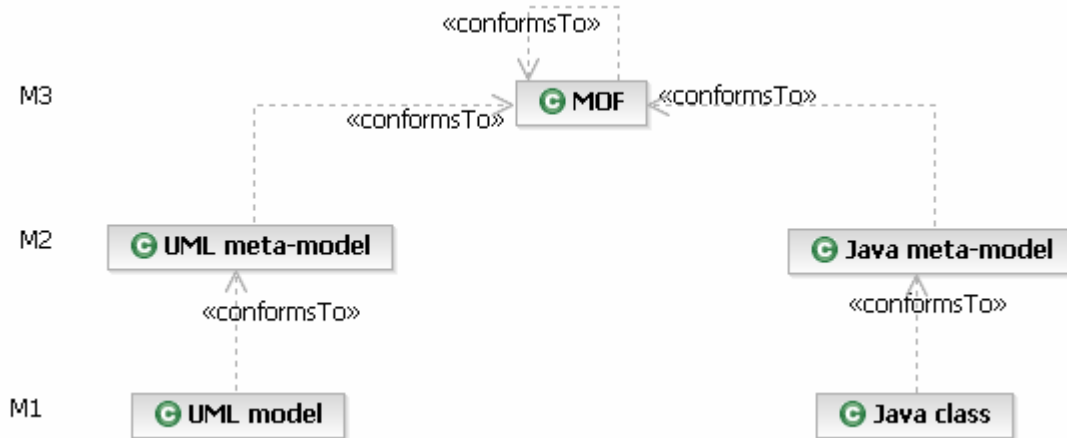
Figure 1 3-level meta-model architecture
