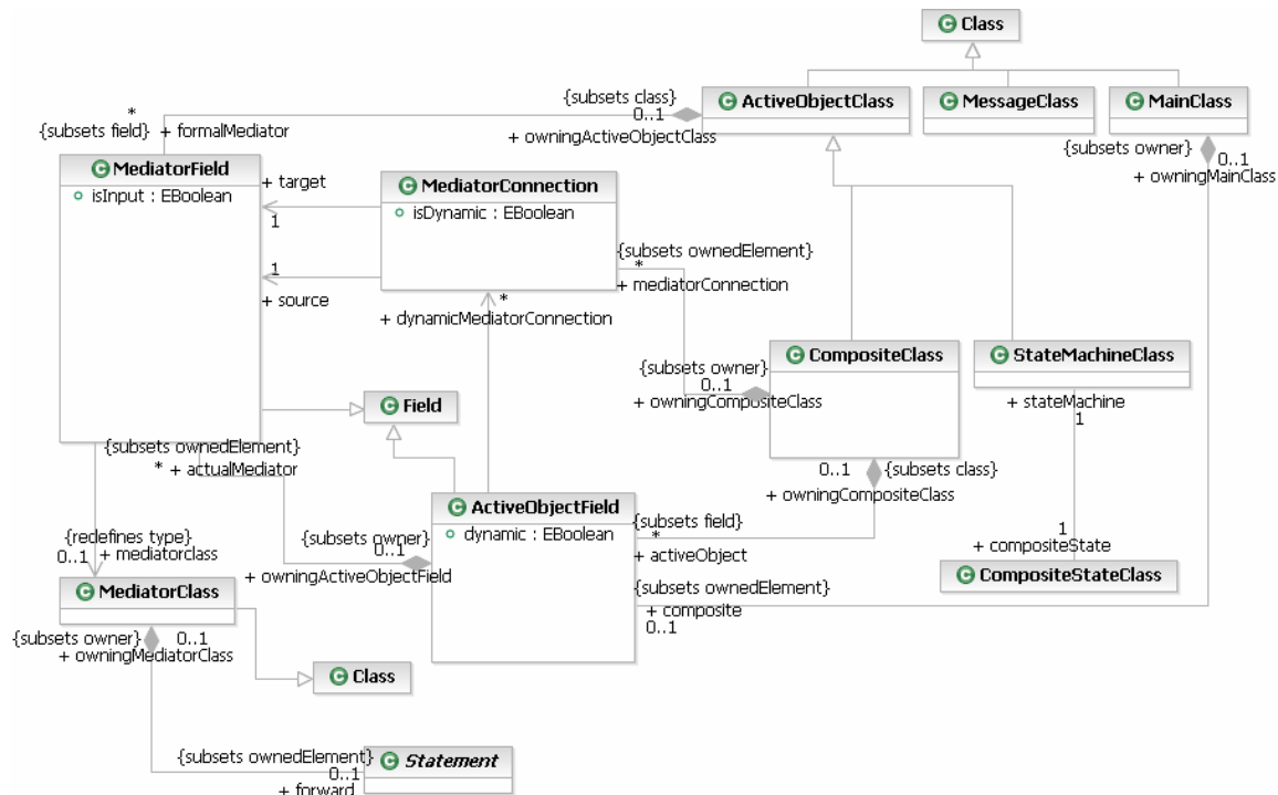
Figure 11 The structure of the JavaFrame extension to the Java meta-model
