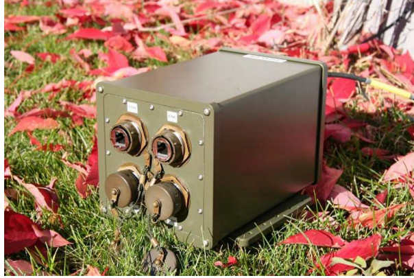
Figure 2.1.: The Intelligent Tactical IP Router designed by Thales is based on a ruggedized PC/104 platform offering four Ethernet ports, two serial ports, one X.25 port and two USB ports [28].
