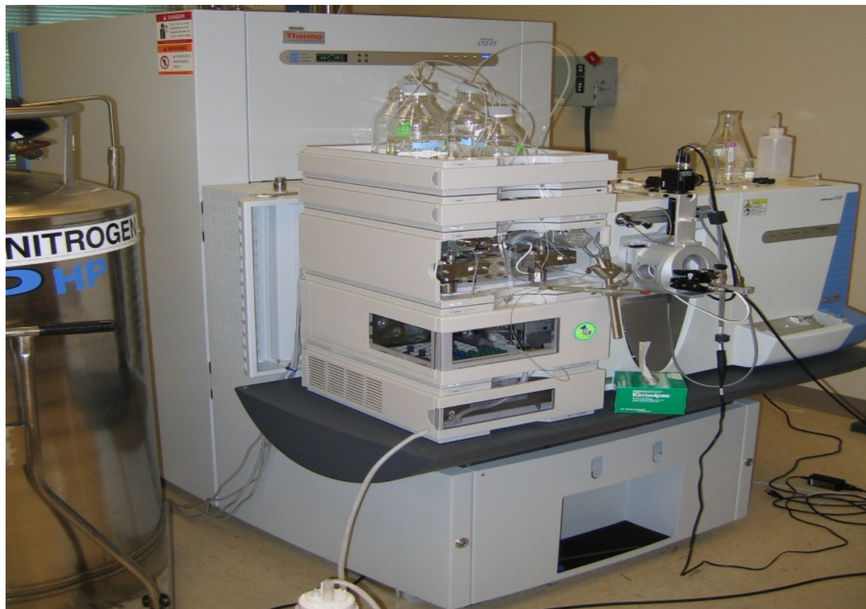
Figure 3.2: LTQ-FT MS interfaced with Agilent 1100 capillary liquid chromatography (Ron Orlando's Lab., CCRC, University of Georgia).
