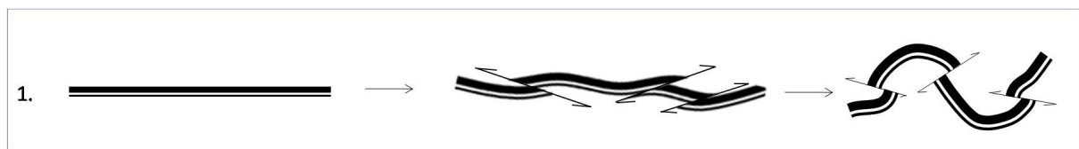
Figure 7.1: 1) Schematic illustration displaying the assumed evolution of structures related to deformational phase 1 associated with bedding-parallel shortening.
