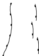
Fig. 4.5 Schematic map view of a continuous fault (left) and a system of segmented faults (right). The left figure displays the master fault as it is defined in this study. Although depicted as a continuous structural feature, some indications of segmentation are present (see text for details).
