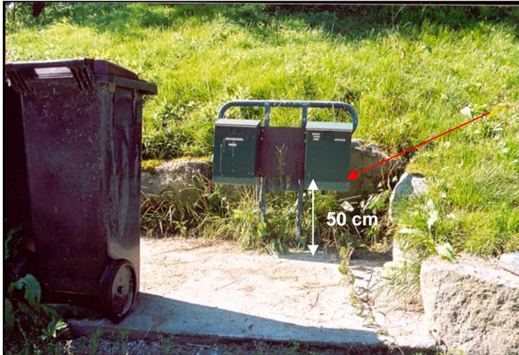
Figure 2.24 Mudmarks on the postboxes at Øygardsneset show thickness of the mud deposit 1 km downstream the fan. For location see Figure 2.1.
