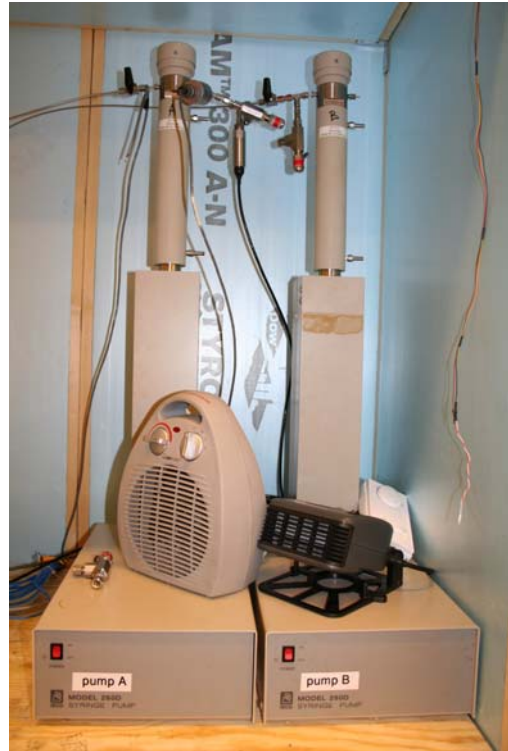
Figure 7: The two syringe pumps used for fluid transport through the claystone.
