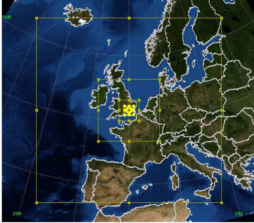
Figure 3.6: Four of the five nested domains that are used in all simulations. All domains are centered over London at approximately (51.5^\circ\text{N}, -0.128^\circ\text{W}) . (Figure from WRF Domain Wizard).
