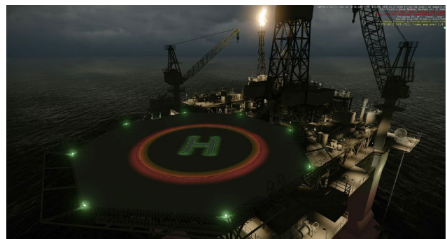
Figure 9. Screen capture from a game engine. The circle of lights was changed during the user meeting to visualize the helicopter pilot's idea about light colour codes.
