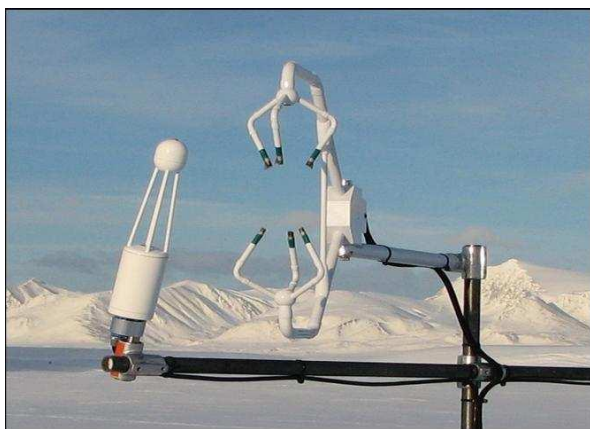
Figure 1.8: Close up view (facing north) of the Bayelva EC system mounted on Leirhaugen hill with the sonic in the center and the IRGA on the left side of the image. Photograph adopted from Westermann (2010).
