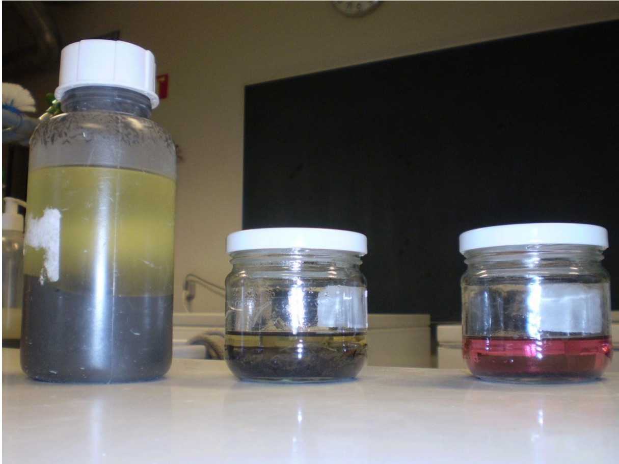
Figure 8 Meiofauna samples before and after the centrifugation; left: in ethanol preserved sample before a centrifugation, middle: >500\mu\text{m} fraction in ethanol after the centrifugation, right: the meiofauna fraction in ethanol+rose bengal (just the thin layer on the bottom)
