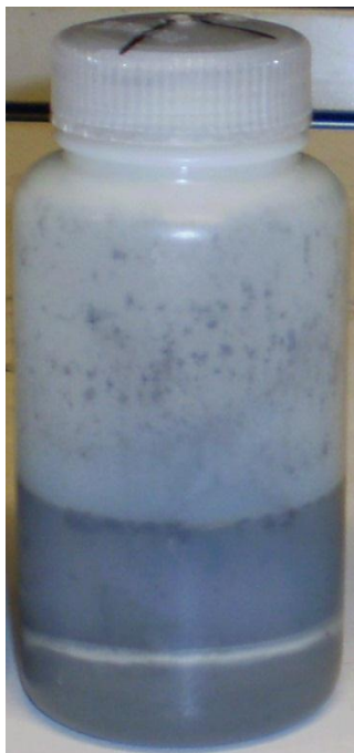
Figure 7 Centrifugation flask after a centrifugation; sediment in the bottom, covered by the white kaolin clay and the liquid levasil on top. Detritus parts can be seen floating on the levasil
