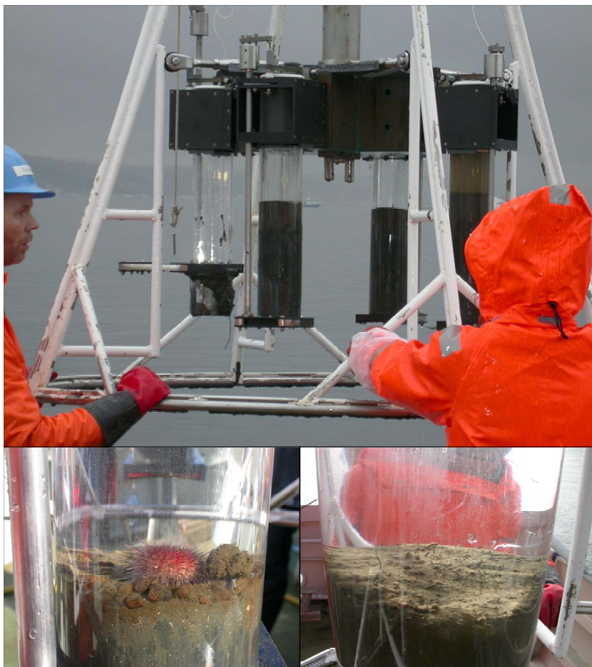
Figure 4 Top picture shows the UiO multicorer used for sediment and faunal sampling. Below are two pictures of the multicorer tubes with sediment samples. The left shows a sample from the green/turquoise acoustic class area with gravel, rocks and a sea urchin. The right one is from the blue acoustic class area, soft sediment with no gravel and worm tubes.
