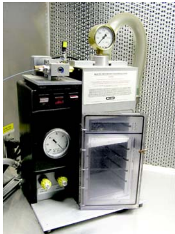
Figure 2-2: The PSD-1000/He Particle Delivery System. An elemental particle of heavy metal is coated with plasmid DNA and shot by micro projectile bombardment into the chloroplast of the agar plated cells. Picture from: http://en.wikipedia.org/wiki/Gene_gun .
