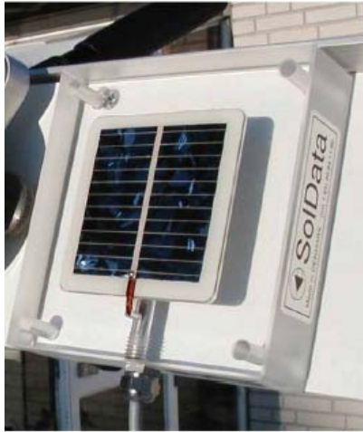
Figur 3. 13: SolData pyranometer (modellnummer 459SPC).
