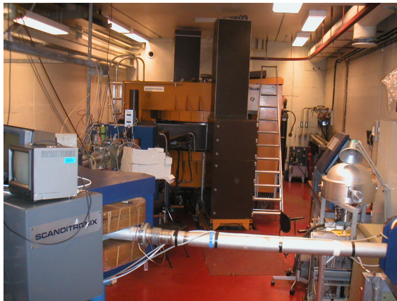
Figure 2.1: The Oslo Cyclotron with the analysing magnet to the left.
