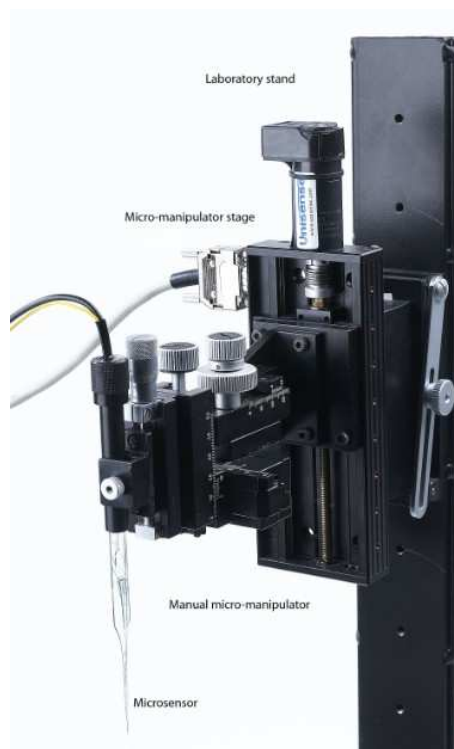
Figure 3.8: The oxygen probe mounted on the micromanipulator (Unisense, Denmark). Picture from www.unisense.com .
