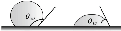
Figure 1.2: Two droplets of different fluids are deposited on a solid surface, surrounded by a gas. The left droplet has a contact angle \theta_w > 90^\circ and is non-wetting, whereas the droplet to the right has a contact angle \theta_w < 90^\circ and is wetting the solid surface.
