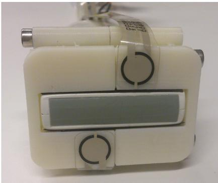
(b) Probe collar with force sensors from the front
