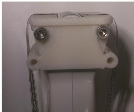
(c) Probe collar with force sensors from the side
