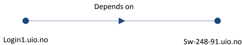
Figure 3.4: graph representation of the connection characteristics of a server and a switch
