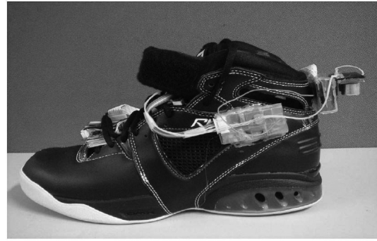
Figure 1.11: Shoe with integrated sensors in [67].
