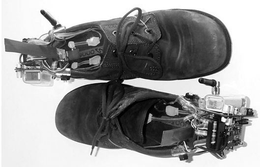
Figure 1.10: Shoe with integrated sensors in [64].
