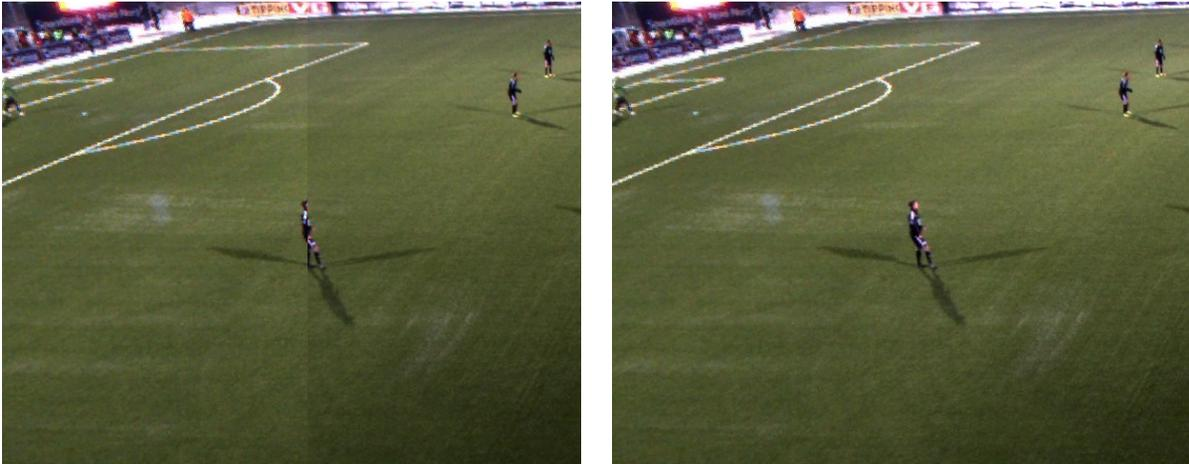
(a) The original stitch pipeline in [10] and [2]: a fixed cut stitch with a straight vertical seam, i.e., showing a player getting distorted in the seam. (b) The new stitch pipeline: a dynamic stitch with color correction, i.e., the system search for a seam omitting dynamic objects (players).
