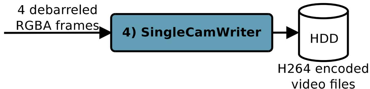
Figure 4.6: The SingleCamWriter module
