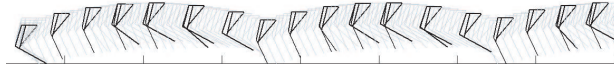
Figure 6.3: Optimal gaits based on jumping. Most efficient gait obtained, but in real life this gait has many drawbacks (E.g. the slippery effect in the floor to feet friction when the robot kicks hard).
