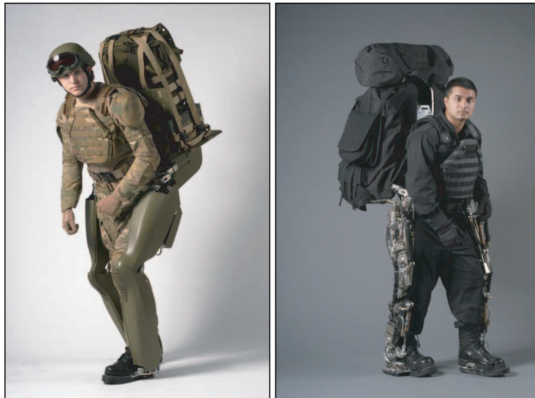
Figure 2.8: Strap-on robotic pants, intended to help soldiers or fire fighters carry heavy loads for long distances.
