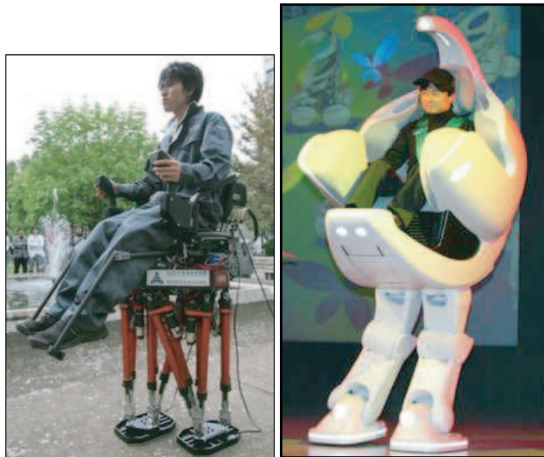
Figure 2.7: Left picture, Waseda University in Tokyo, Japan, have made a walking robot-chair, applicable where wheelchairs don't reach. Right picture shows Toyota's "I-foot", controlled by a joystick inside.
