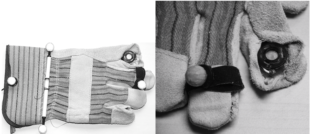
Figure 3.8 The vibrotactile glove with index finger actuator exposed. On the right, a closeup of the index finger actuator.
