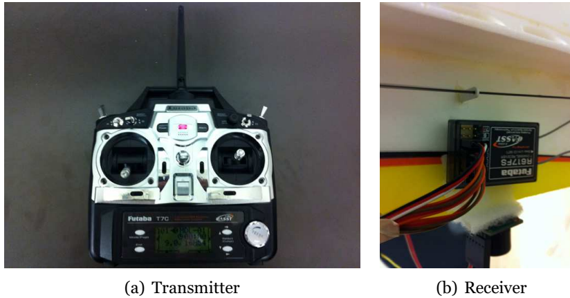
Figure 4.5: 7 channel Futaba RC system
