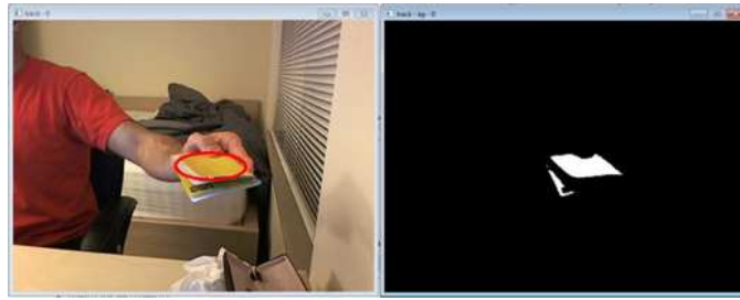
Figure 4.17: 2D tracking based on colour thresholding
