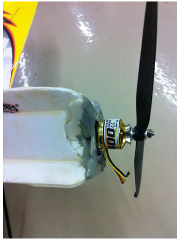
Figure 4.3: Reinforcement of the motor mount
