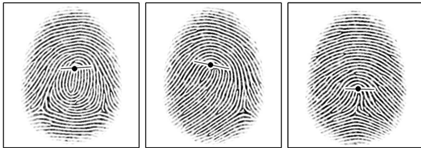
Figure 3.21: Cores and principal directions of fingerprints of types whorl, loop and tented arch
