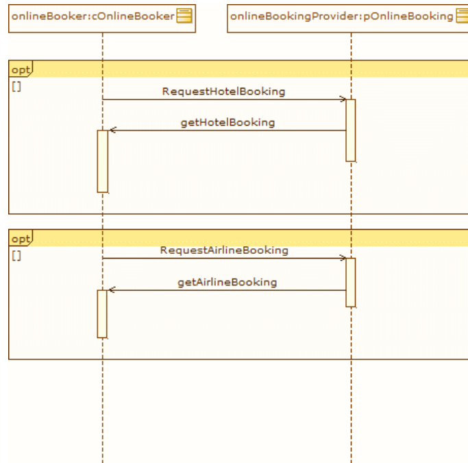
Figure 5.16: UML interaction diagram detailing a protocol between an onlineBooker and an onlineBookingProvider
