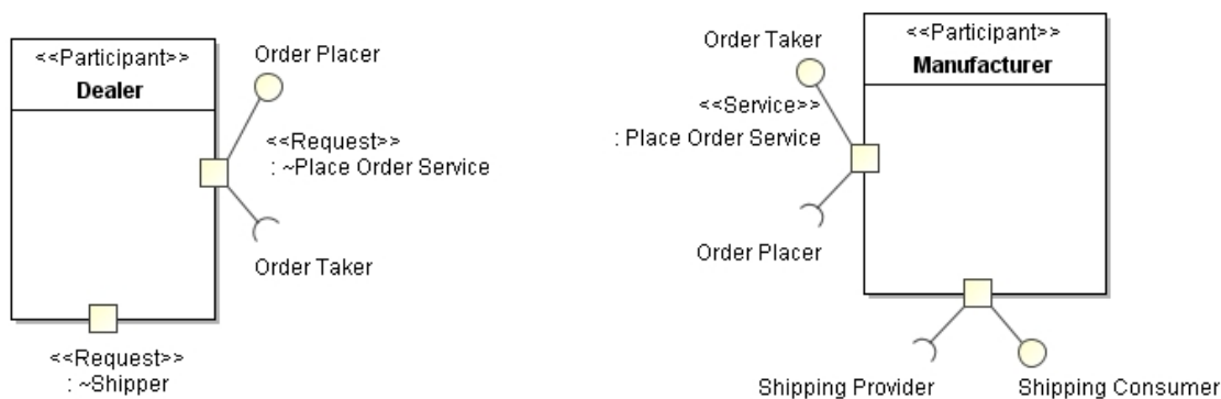
Figure 5.13: Participating in Service - The use of conjugate (tilde) naming for opposite service interfaces
