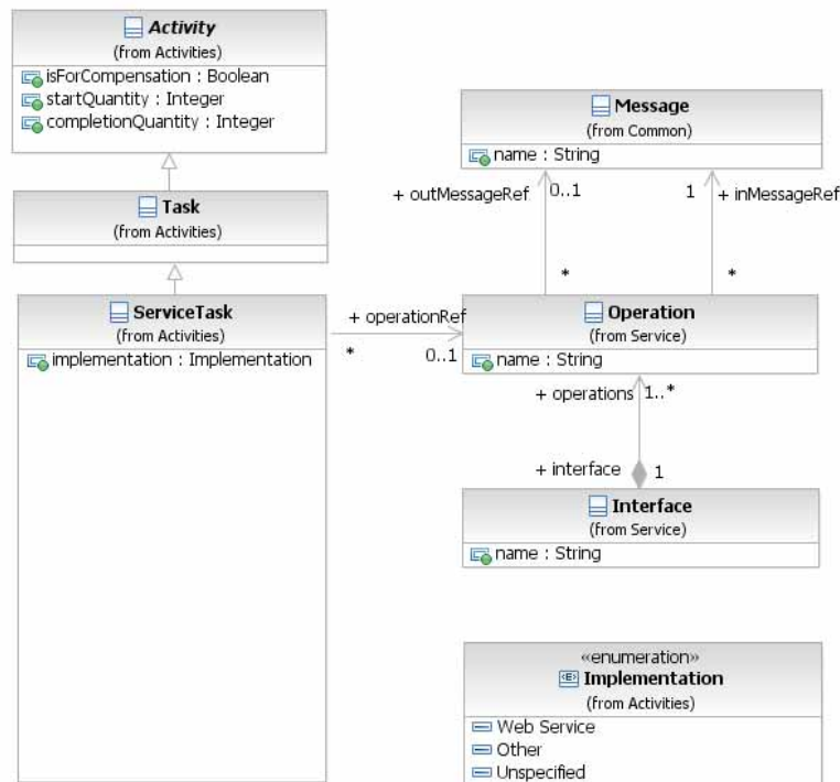
Figure B.9: BPMN 2.0 ServiceTask class diagram
