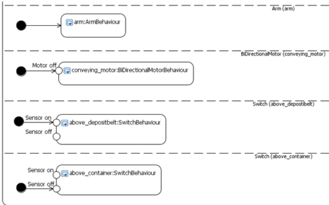
Figure 102 - Detailed view of Crane part regions from state machine diagram in Figure 100.
