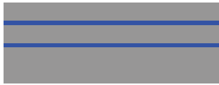
(a) The starting point is a DSOI wafer with 10\mu\text{m} thick device layers and 2\mu\text{m} BOX
