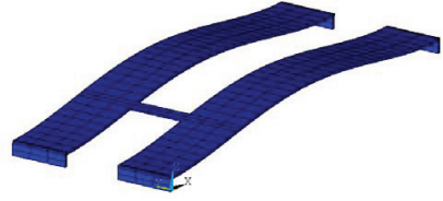
(b) Perspective view of a filter from two vertical bending mode resonators coupled via a small bar. Electrodes underneath each double clamped bar function as input and output electrodes for the electrostatic actuation. Example structure from [67]
