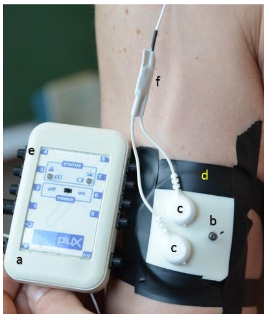
Figure 9. The electrode, connectors, amplifier, and wires.
