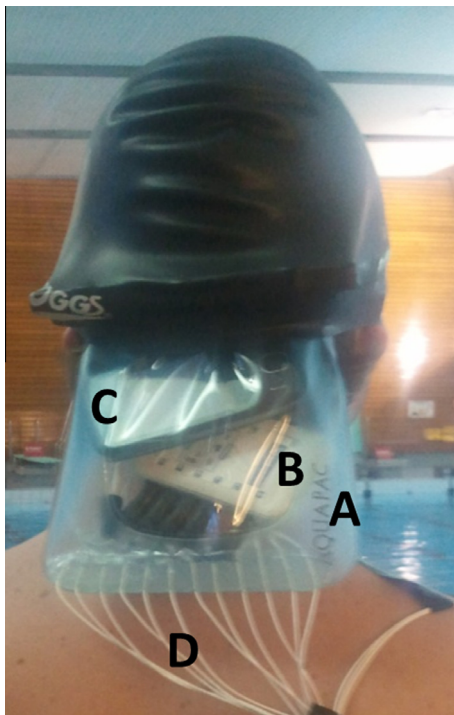
Fig. 3. The waterproof pouch. Legend: (A) waterproof pouch; (B) input box; (C) data logger; and (D) cables (coming from the EMG sensors).
