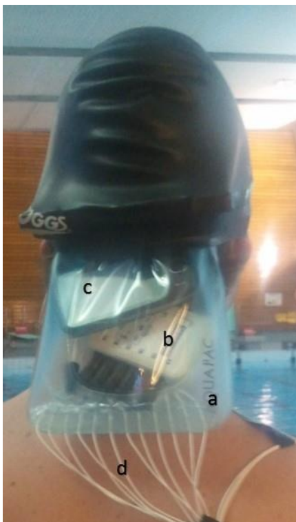
Figure 10. The waterproof pouch for electromyographic testing in water. (a) waterproof pouch; (b) input box; (c) data logger; and (d) cables (coming from the EMG sensors).
