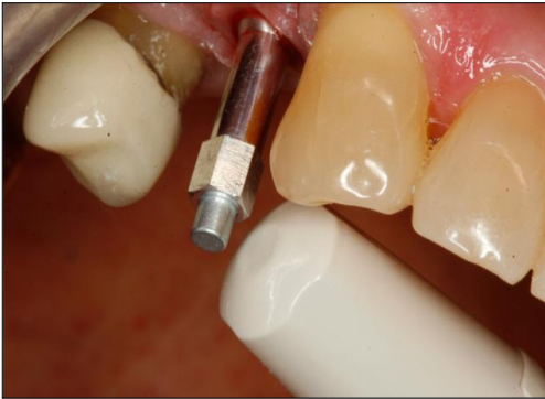
Figure 15. Resonance frequency analysis using the Osstell mentor® (Osstell AB, Gothenburg, Sweden) with the SmartPeg™ inserted into the implant and directing the Osstell® probe against the peg at four different directions to achieve the lowest ISQ value which then was recorded.
