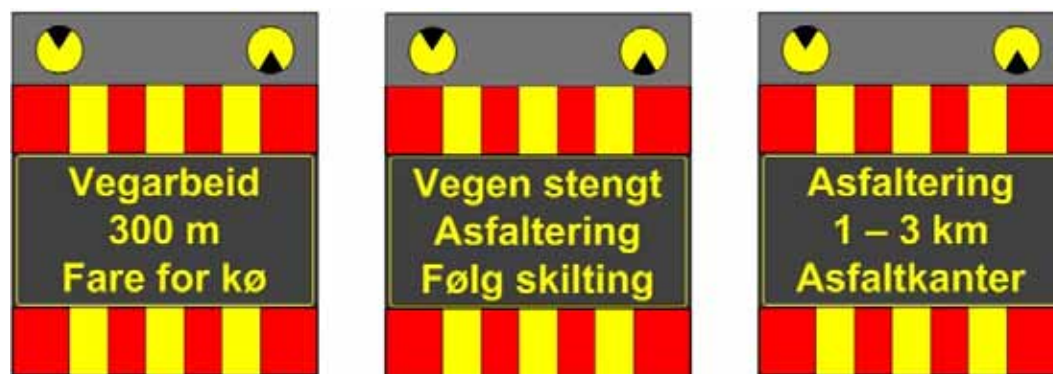
Figure 3.2.4 Examples of sign 560 on warning panels
