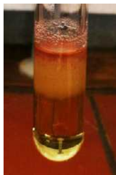
Figure 2.19: Purple metallic gold clusters trapped in polymer beads.
