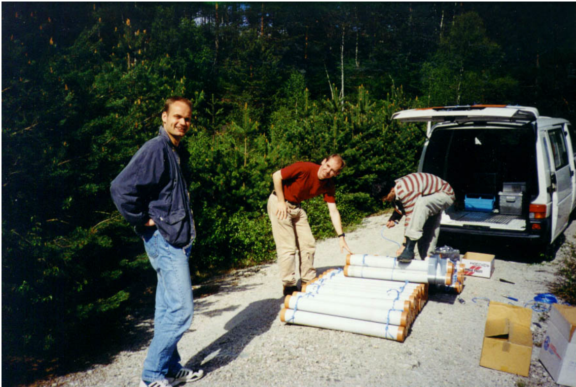
Figure 4. Each single PVC pipe contained 12.17 kg of dynamite. The pipes were tied together in bundles of 3-4 pipes each. To every bundle 1200 grams of extra dynamite and a detonator of 250 grams were attached. From left to right: Benny Bruun, Andy Ross and Michel Heeremans. Phot by Annik Myhre
