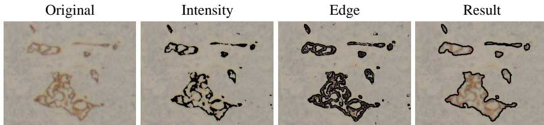
Figure 3.6: Global Threshold: The black and white result obtained from the intensity image at step 3, and the gradient image at step 4, superimposed on the original image. To the right the perimeter of the final result is shown. Uncropped final images (not just the perimeter) are shown in figure 4.14
