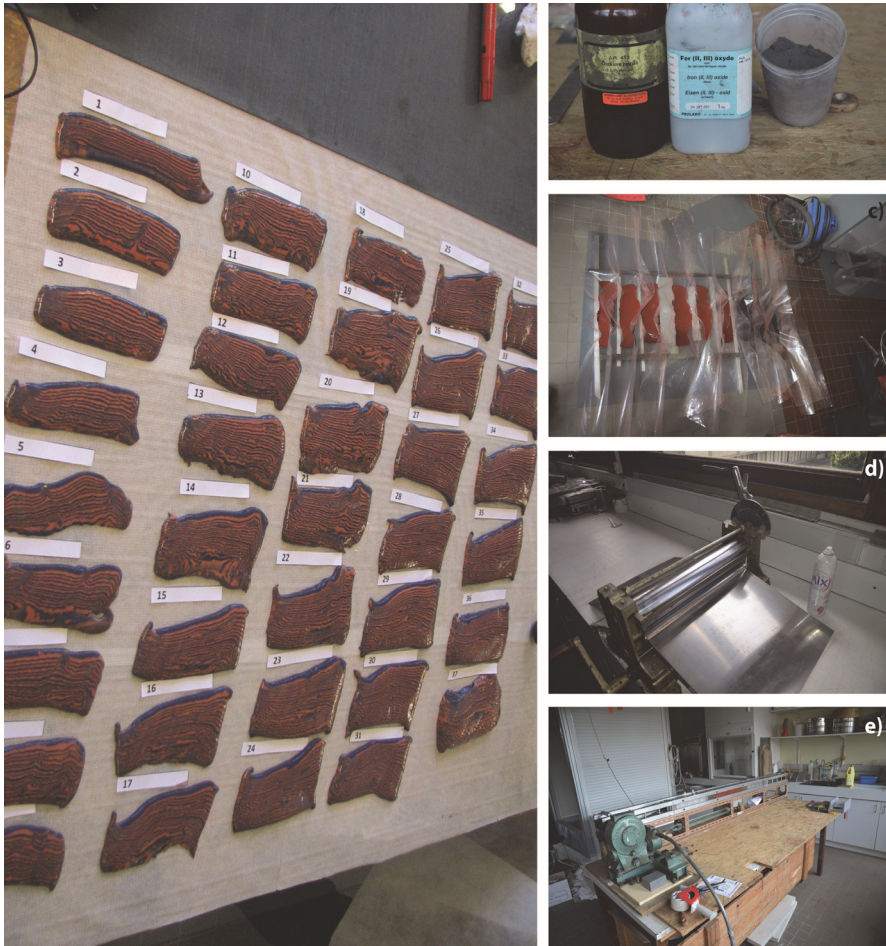
Figure 8: a) Sections cut from the deformed model. The reconstruction of the models was not based on pictures of the extracted cross-sections but on pictures of the sections when they were still in the machine. b) Oleic acid and iron oxide used to change the viscosity of the silicon. c) Silicones resting to release air bubbles after the mixing with oleic acid, iron oxide, and sand. d) Double roll device used for the layer production. This rolling device is from a bakery where it was used to produce butter dough. e) Simple shear machine used for the experiments. The machine has a total length of approximately 2.5 meters.
