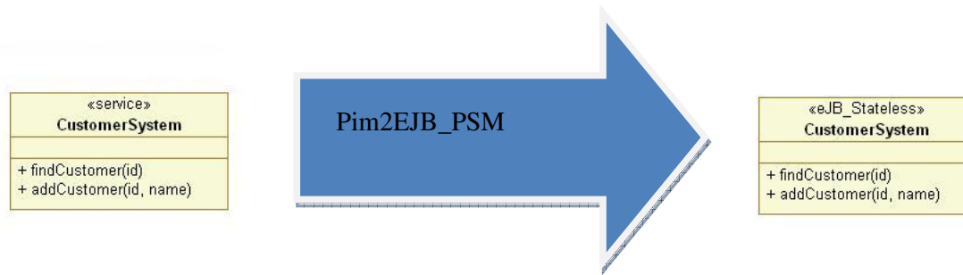
Figure 7: Illustration of the model to model transformation of the class Customer System .
